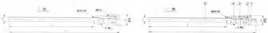
1. 侧帽 Valve bonnet 2. O-Ring 3. 气门芯 Valve inside 4. 阀体 Valve body 5. 铜接管 Copper tube
