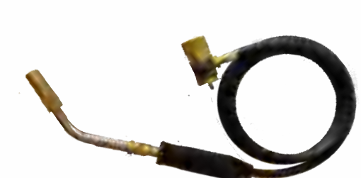
Gas Type: MAPP/Propane/LPG Connection Standard: CG600 Max Flame Temperature: > 3600°F(MAPP Gas) Soft Solder: Max.Φ4" Brazing: Max.Φ1 1/4"
