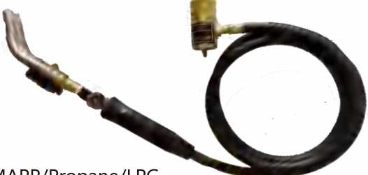
Gas Type: MAPP/Propane/LPG Connection Standard: CG600 Max Flame Temperature: > 3600°F(MAPP Gas) Soft Solder: Max.Φ4" Brazing: Max.Φ1 1/4"
