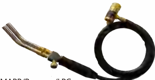
Gas Type: MAPP/Propane/LPG Connection Standard: CG600 Max Flame Temperature: > 3600°F(MAPP Gas) Soft Solder: Max.Φ4" Brazing: Max.Φ1 1/4"
